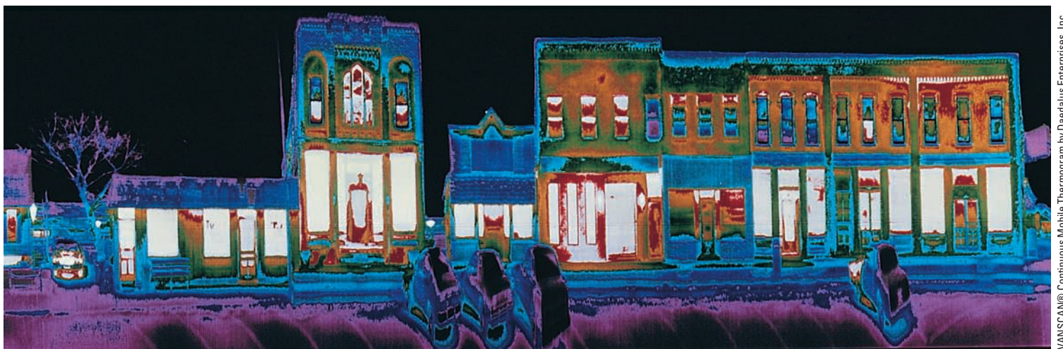
Figure 13-23 A thermogram , or infrared photo, showing heat loss (red, white, and orange) around the windows, doors, roofs, and foundations of houses and stores in Plymouth, Michigan (USA). Many homes and buildings in the United States and other countries are so full of leaks that their heat loss in cold weather and heat gain in hot weather are equivalent to what would be lost through a large window-sized hole in a wall of the house. Question: How do you think the place where you live would compare to these buildings in terms of heat loss?
