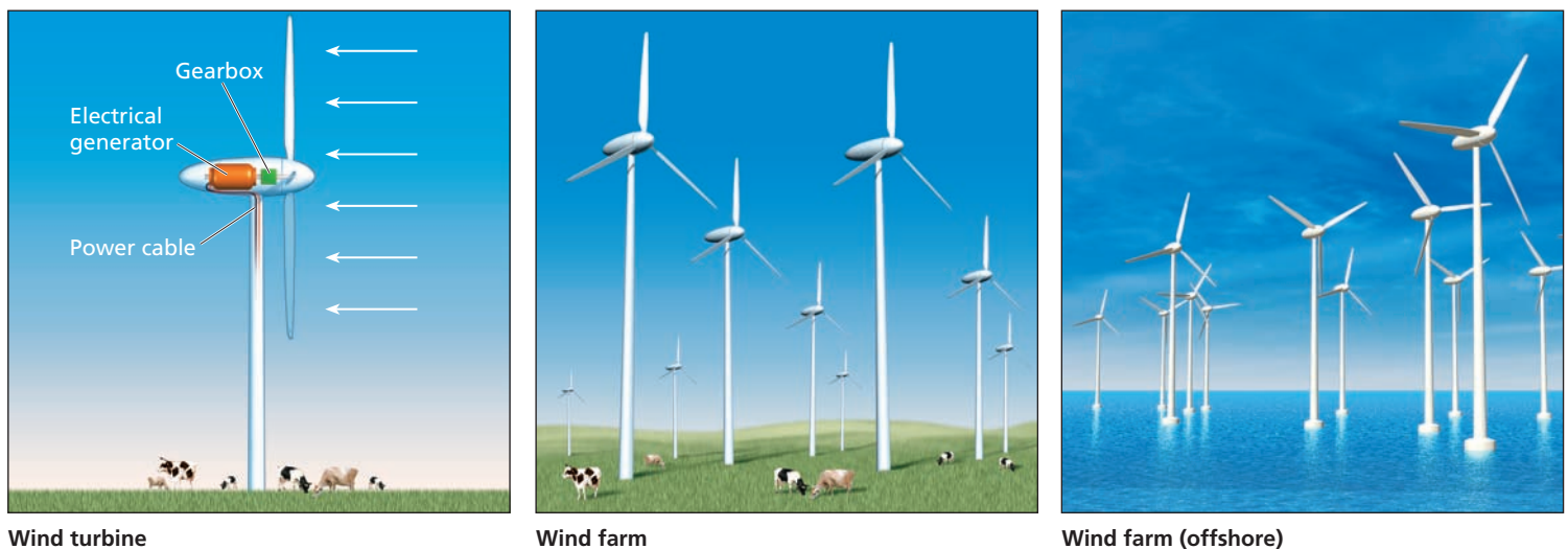
Figure 13-33 Solutions: A single wind turbine (left) can be used to produce electricity. Increasingly, they are being used in interconnected arrays of ten to hundreds of turbines. These wind farms or wind parks can be located on land (middle) or offshore (right). Land lying under these turbines can still be used to grow crops or raise cattle.
