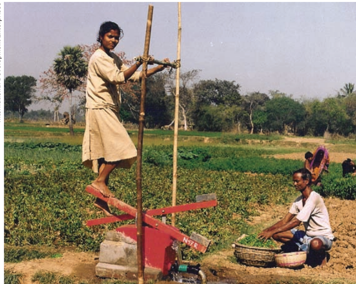
Photo 7 Treadle pump used to supply irrigation water in parts of Bangladesh and India.
