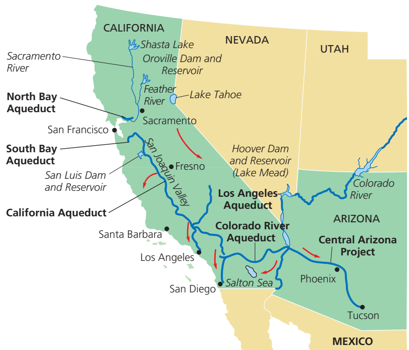
Figure 11-12 California Water Project and the Central Arizona Project. These projects involve large-scale water transfers from one watershed to another. Arrows show the general direction of water flow.
