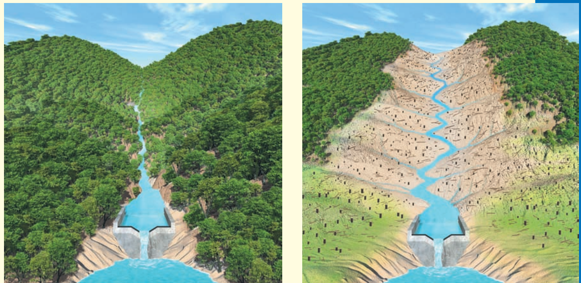
Figure 2-1 Controlled field experiment to measure the effects of deforestation on the loss of water and soil nutrients from a forest. V-notched dams were built at the bottoms of two forested valleys so that all water and nutrients flowing from each valley could be collected and measured for volume and mineral content. These measurements were recorded for the forested valley (left), which acted as the control site. Then all the trees in the other valley (the experimental site, right) were cut and the flows of water and soil nutrients from this experimental valley were measured for 3 years.
